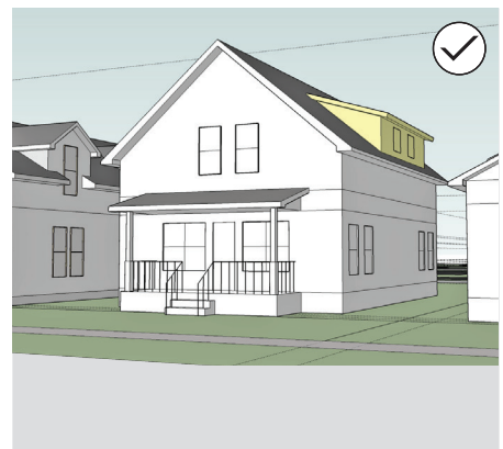
Figure 23: Location & Design of a Residential Addition
