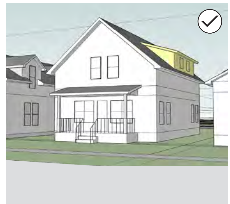
Figure 23: Location & Design of a Residential Addition
